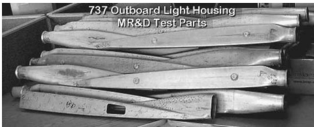
Fig. 11 Phase II SPF light housing test demonstration parts
