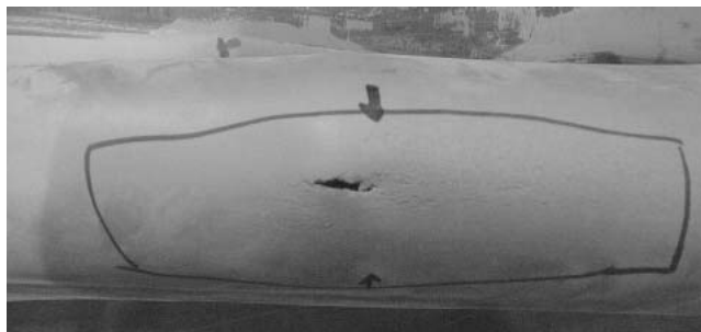
Fig. 14 Close-up of cavitation failure in early seamless tube
