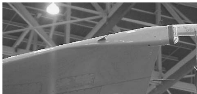
Fig. 1 Outboard light housing, installed on the wing of the Boeing 737NG aircraft
