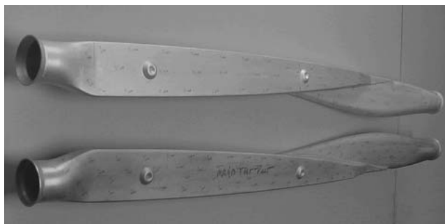
Fig. 15 Al 5083 superplastically formed seamless tube test parts
